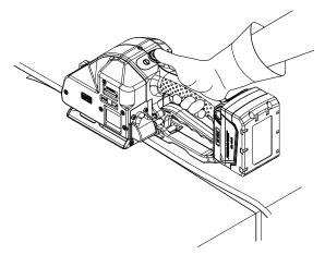
The plastic strap is welded and cut off from the rest of the strap.
